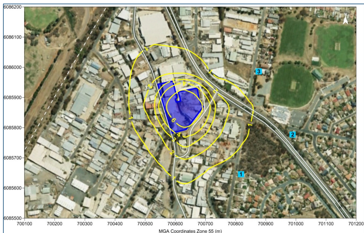
Figure 1: Predicted 99 th percentile nose-response average ground level odour concentrations – Scenario 1, with proposed mitigation measures
