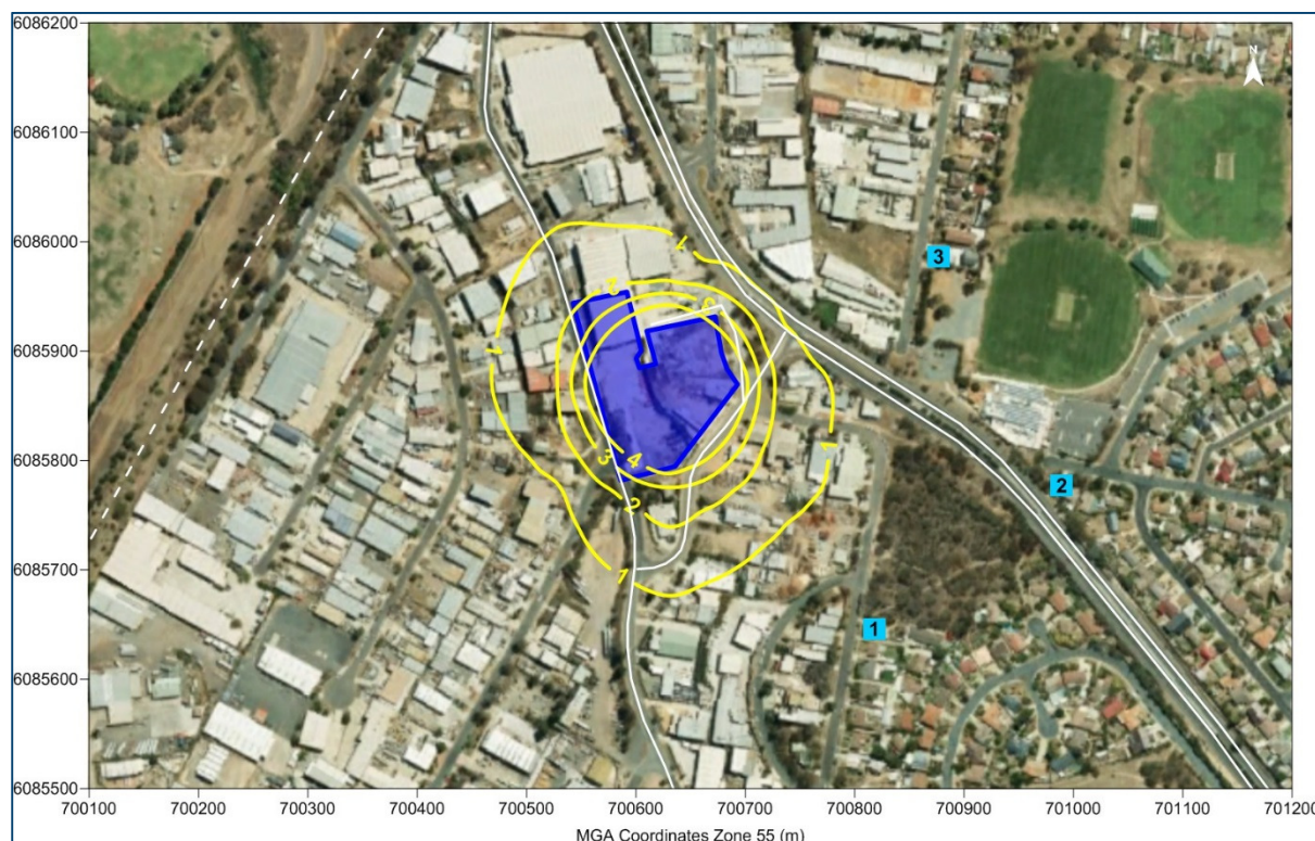
Figure 2: Predicted 99 th percentile nose-response average ground level odour concentrations – Scenario 2, with filtration odour management system
